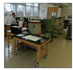
Countroom (2902) - Gamma-Spec system w/HPGE detectors, Zhong Zhang at APEX console.
