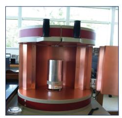
Ultra-high efficiency HPGe Detector No. 1 (with open shield) - Radiochemistry Countroom
